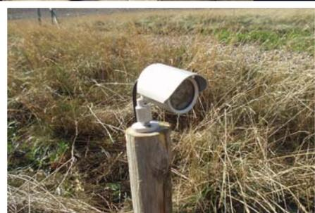
The cameras used to monitor the nesting birds are based on security cameras, a market that has produced high quality cameras at a low cost. The cameras used to monitor the beach under storm conditions are security cameras with additional protection, but are proving difficult to keep working during the extreme weather encountered on Chesil Beach.
